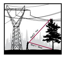
\*If you can't see all 3 points from one location or you have a TruPulse 200 model, measure the height of the tree from one spot and then start the ML routine over again to get the distance to the wire in steps 4 and 5. Follow the proper procedure for obtaining accurate ML - SD values with your instrument.
